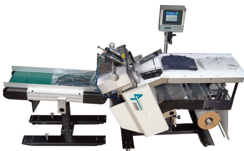
Bulky or lightweight products are difficult to package in a traditional, vertical bagger. Davida manually slides product (shirts, left; sponges, right) toward an open bag.
